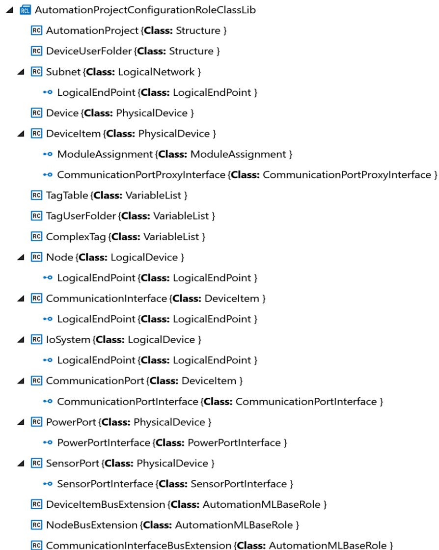
Figure 17 – AutomationProjectConfigurationRoleClassLib in AutomationML Editor view
